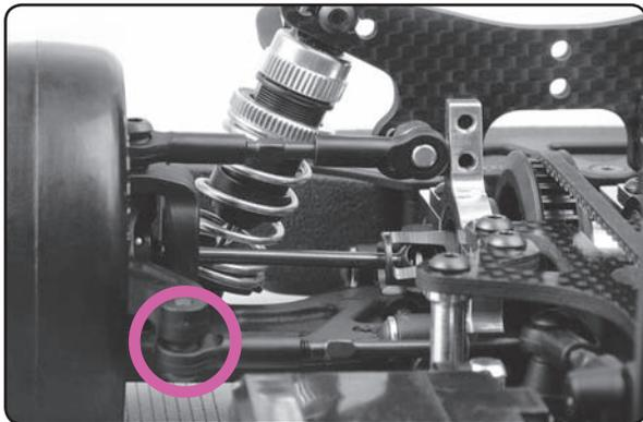
Bump steer is an undesirable handling effect that occurs when a car's front toe angle changes as its suspension compresses or rebounds, from the position that was pre-set using a setup station.
