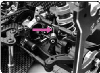
IMPORTANT: ADJUST TWEAK USING ANTI-ROLL BARS ONLY AFTER YOU HAVE ADJUSTED TWEAK USING SPRING PRELOAD.
