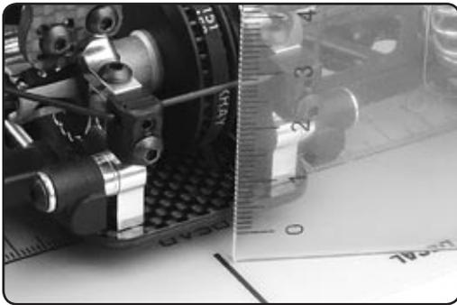
3. Place the ruler vertically beside the chassis, so that you can see how much distance there is between the flat surface and the bottom of the chassis.
