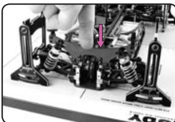
4. Push down and release the front and rear of the car so that the suspension settles.
