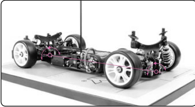
A “roll center” is a theoretical point around which the chassis rolls, and is determined by the design of the suspension. Front and rear suspensions normally have different roll centers. The “roll axis” is the imaginary line between the front and rear roll centers.
