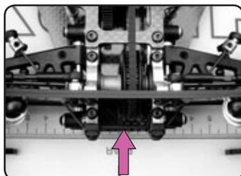
9. Attach the rear anti-roll bar.
