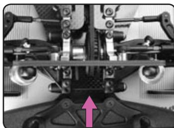
10. Attach the front anti-roll bar.
