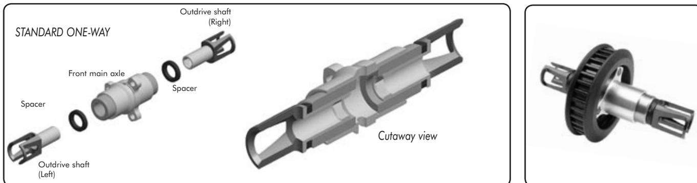
When using an XRAY Multi-Diff™ in “one-way” mode, outdrive shafts (left and right) are not connected to each other, nor to front main axle. This mode combines the characteristics of a solid axle and a differential.
