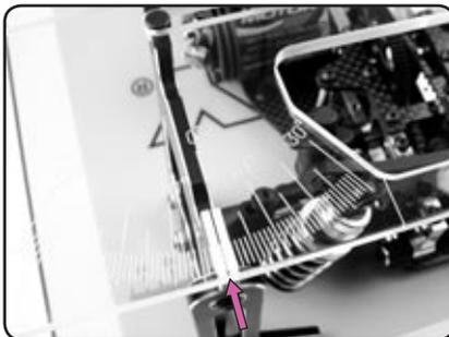
5. To read the toe value of the left rear wheel, push the toe gauge to the right until the pin on the top edge of the left set-up stand hits the edge of the slot in the toe gauge.
