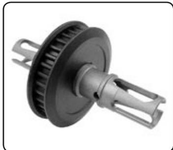
Differentials allow the wheels at opposite ends of the same axle to rotate at different speeds. Why is this important? When a car turns in a circle, the outer wheel has a larger diameter circle to follow than the inner wheel, so it needs to rotate faster to keep up. If the differential is too tight, the result is that the wheels "fight" each other for the proper rotation speed; the result is a loss of traction. Generally, the more grip a track has, the tighter the diff action should be.
