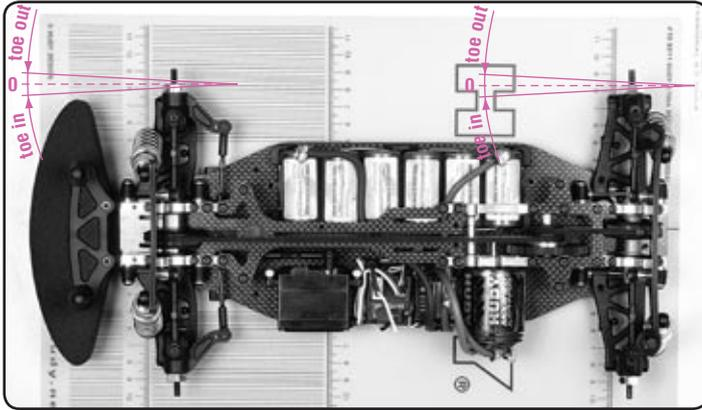
Toe is the angle of the wheels when looked at from above the car. Toe is used to stabilize the car at the expense of traction, as it introduces friction and therefore some slip in the tires.
