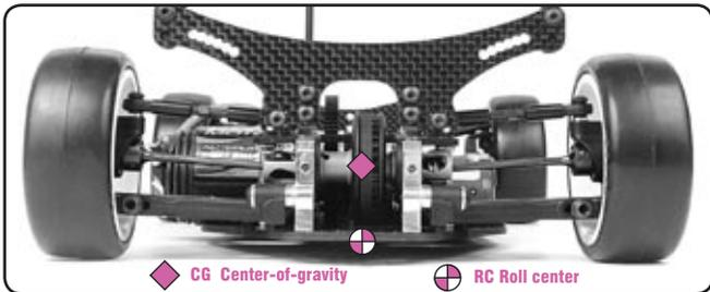
Here are some basic facts about roll center (RC) and center-of-gravity (CG).
