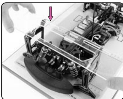
6. To adjust front toe, set the toe gauge atop the front set-up stands and then repeat the procedure.
