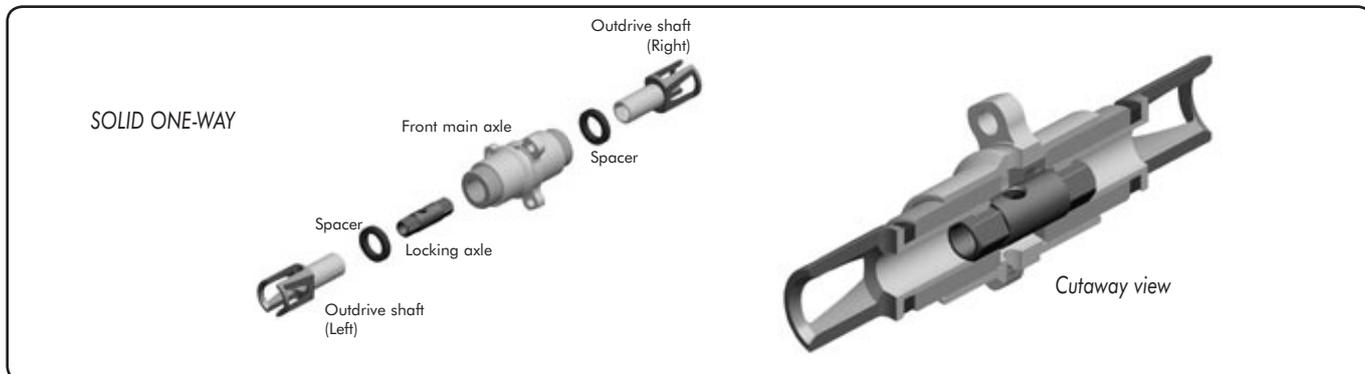
When using an XRAY Multi-Diff™ in “one-way” mode, outdrive shafts (left and right) are not connected to each other, nor to front main axle. This mode combines the characteristics of a solid axle and a differential.
